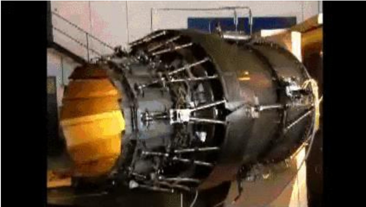
Eurofighter Typhoon thrust nozzle
