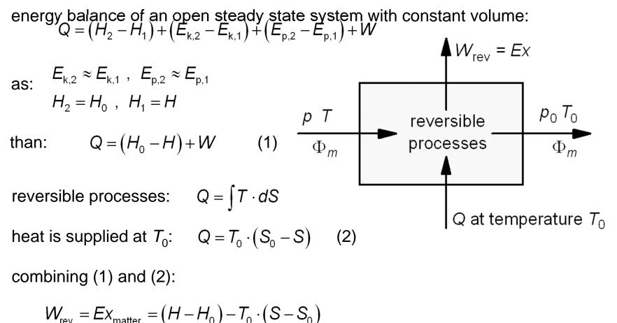
and for a flow of mass:  $\Phi_{W_{rev}} = \Phi_{Ex_{flow}} = \Phi_m \cdot \left[ \left( h - h_0 \right) - T_0 \cdot \left( s - s_0 \right) \right]$
