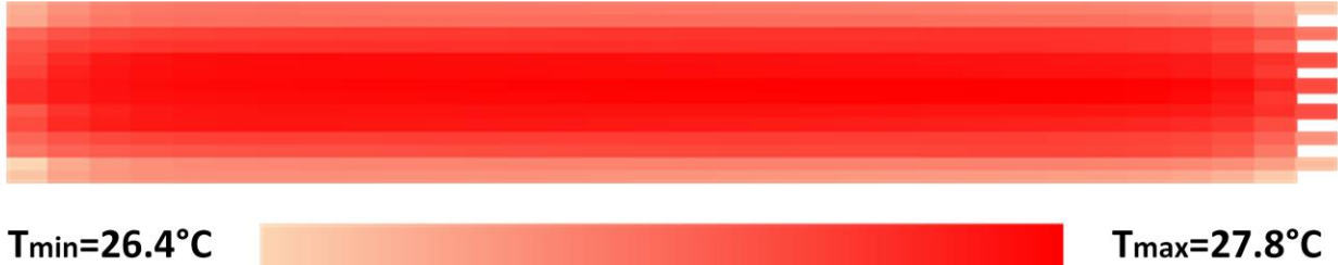
Figure 10: Distribution of highest temperature in each battery cell with counter-flowing coolant; \dot{m}_{cool} = 0.05kg/s , T_{cool,in} = 10^\circ C , R = 5 .
