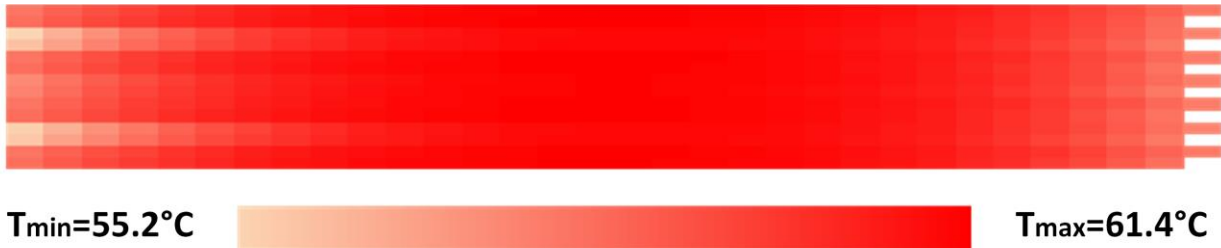
Figure 8: Distribution of highest temperature in each battery cell with counter-flowing coolant; \dot{m}_{cool} = 0.05\text{kg/s} , T_{cool,in} = 10^\circ\text{C} , R = 2 .
