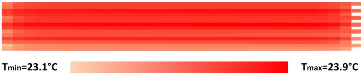
Figure 13: Distribution of highest temperature in each battery cell with counter-flowing refrigerant; \dot{m}_{cool} = 0.006\text{kg/s} , T_{sat} = 10^\circ\text{C} , x_{in} = 0.22 , R = 5 .
