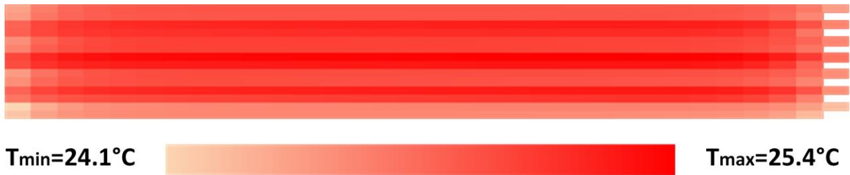
Figure 15: Distribution of highest temperature in each battery cell with counter-flowing refrigerant; \dot{m}_{cool} = 0.006\text{kg/s} , T_{sat} = 10^\circ\text{C} , x_{in} = 0.22 , R \approx 1 .
