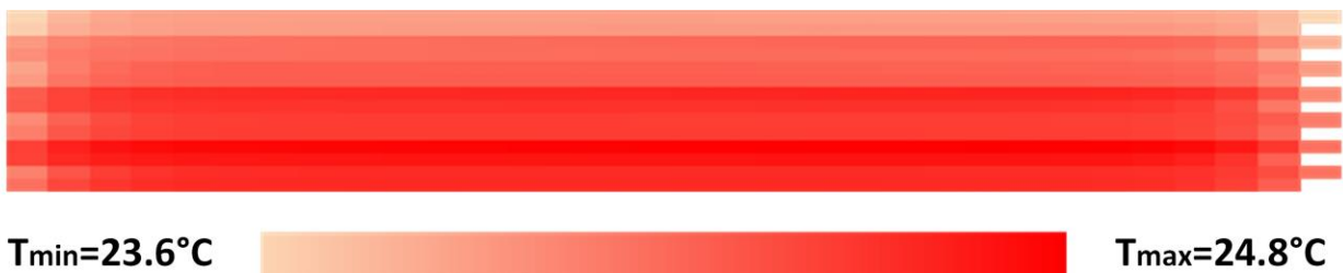
Figure 19: Distribution of highest temperature in each battery cell with counter-flowing refrigerant; the outlet of one cooling tube is connected with the inlet of another tube; \dot{m}_{\text{cool}} = 0.0095\frac{\text{kg}}{\text{s}} , T_{\text{sat}} = 10^\circ\text{C} , x_{\text{in}} = 0.22 , R \approx 1 .
