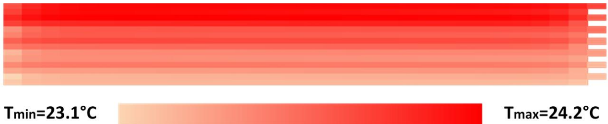
Figure 17: Distribution of highest temperature in each battery cell with parallel-flowing refrigerant; \dot{m}_{cool} = 0.006\text{kg/s} , T_{sat} = 10^\circ\text{C} , x_{in} = 0.22 , R = 5 .
