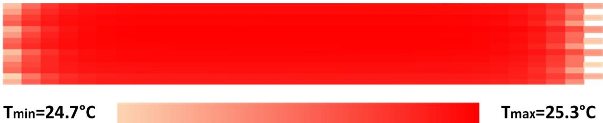
Figure 11: Distribution of highest temperature in each battery cell with counter-flowing coolant; \dot{m}_{cool} = 0.2kg/s , T_{cool,in} = 10^\circ C , R \approx 1 .
