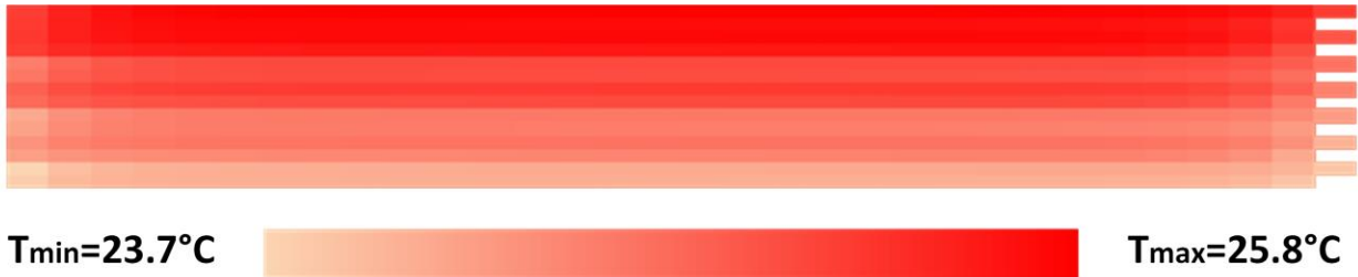
Figure 18: Distribution of highest temperature in each battery cell with parallel-flowing refrigerant; \dot{m}_{\text{cool}} = 0.006\text{kg/s} , T_{\text{sat}} = 10^\circ\text{C} , x_{\text{in}} = 0.22 , R \approx 1 .
