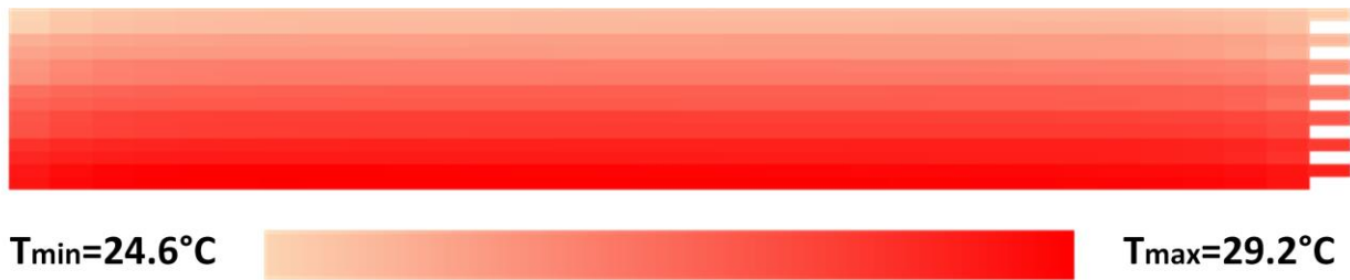
Figure 12: Distribution of highest temperature in each battery cell with parallel-flowing coolant; \dot{m}_{cool} = 0.04\text{kg/s} , T_{cool,in} = 10^\circ\text{C} , R = 5 .
