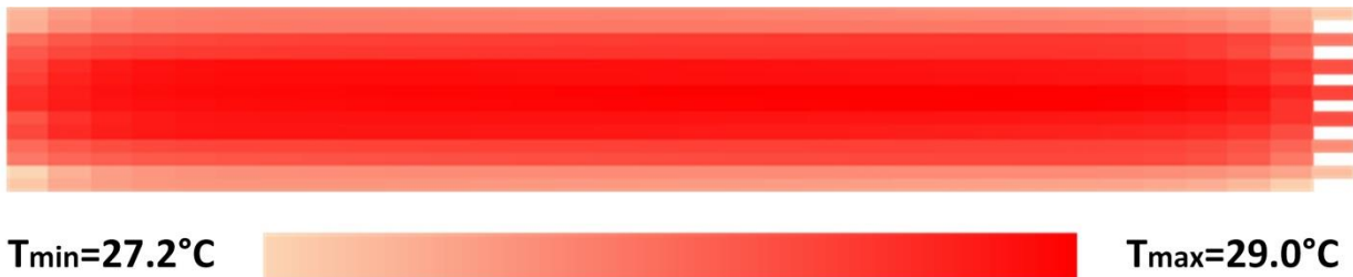
Figure 9: Distribution of highest temperature in each battery cell with counter-flowing coolant; \dot{m}_{cool} = 0.04\text{kg/s} , T_{cool,in} = 10^\circ\text{C} , R = 5 .
